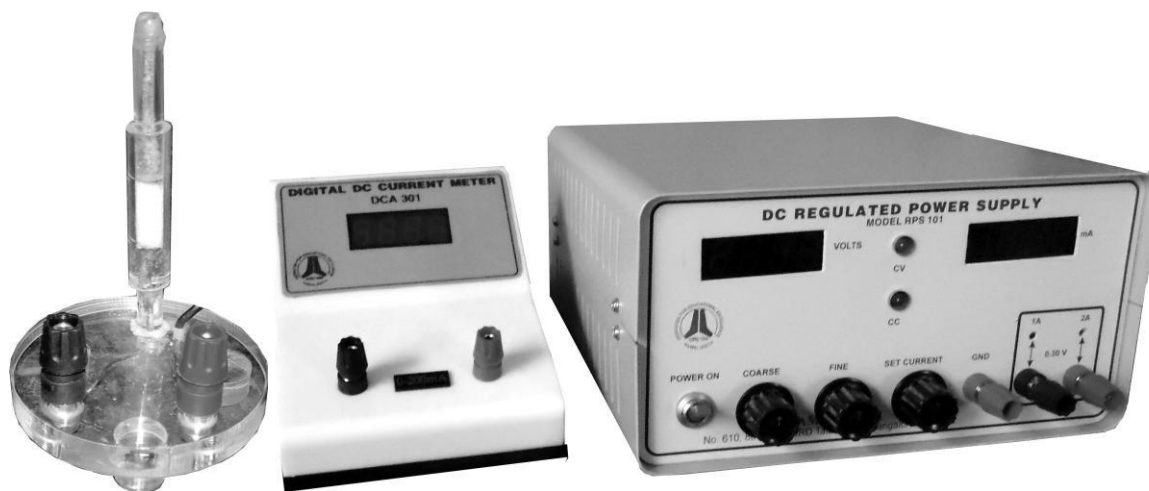
Figure: Resistivity cell and Resistivity measurement setup
